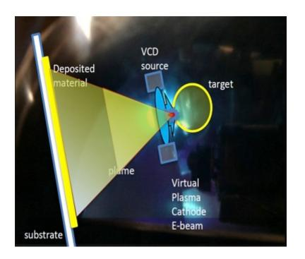
VCD Generates Plume of Carbon Ions from Graphite Target
