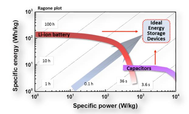
Energy : system's capability to do work [Wh/kg] Power : the rate at which work is performed or energy is converted [energy/time], [W/kg]
