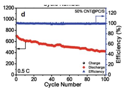
Specific capacity and coulombic efficiency retentions of 50% CNT@PC/S composite for 100 cycles at scan rate 0.5 C,
