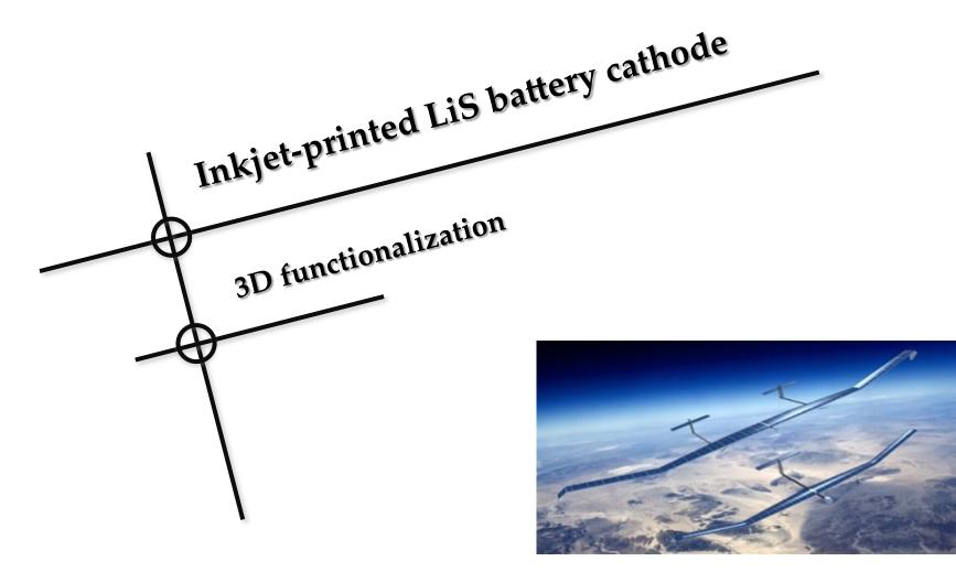
The Zephyr 7 holds the official endurance record for an unrefueled flight, lasting 336 hours, 22 minutes and 8 seconds. It uses sunlight to charge a lithium-sulfur battery during the day.
