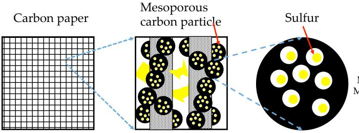
Micropores: 1-10 nm Mesopores: 10-100 nm
