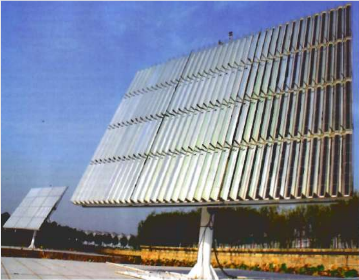
Shanghai: Part of a 100 kW 3 rd project completed last year by US-based JX Crystals Inc. at the Shanghai Flower Port. Low-concentration systems account for the majority of CPV installed to date.
