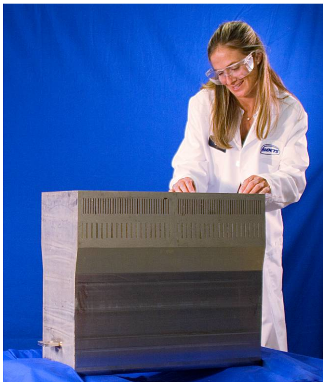
1/3 scale SMR reactor Device: 550mm x 300mm x 600mm Capacity if operated: 9,350 m 3 /day H 2
