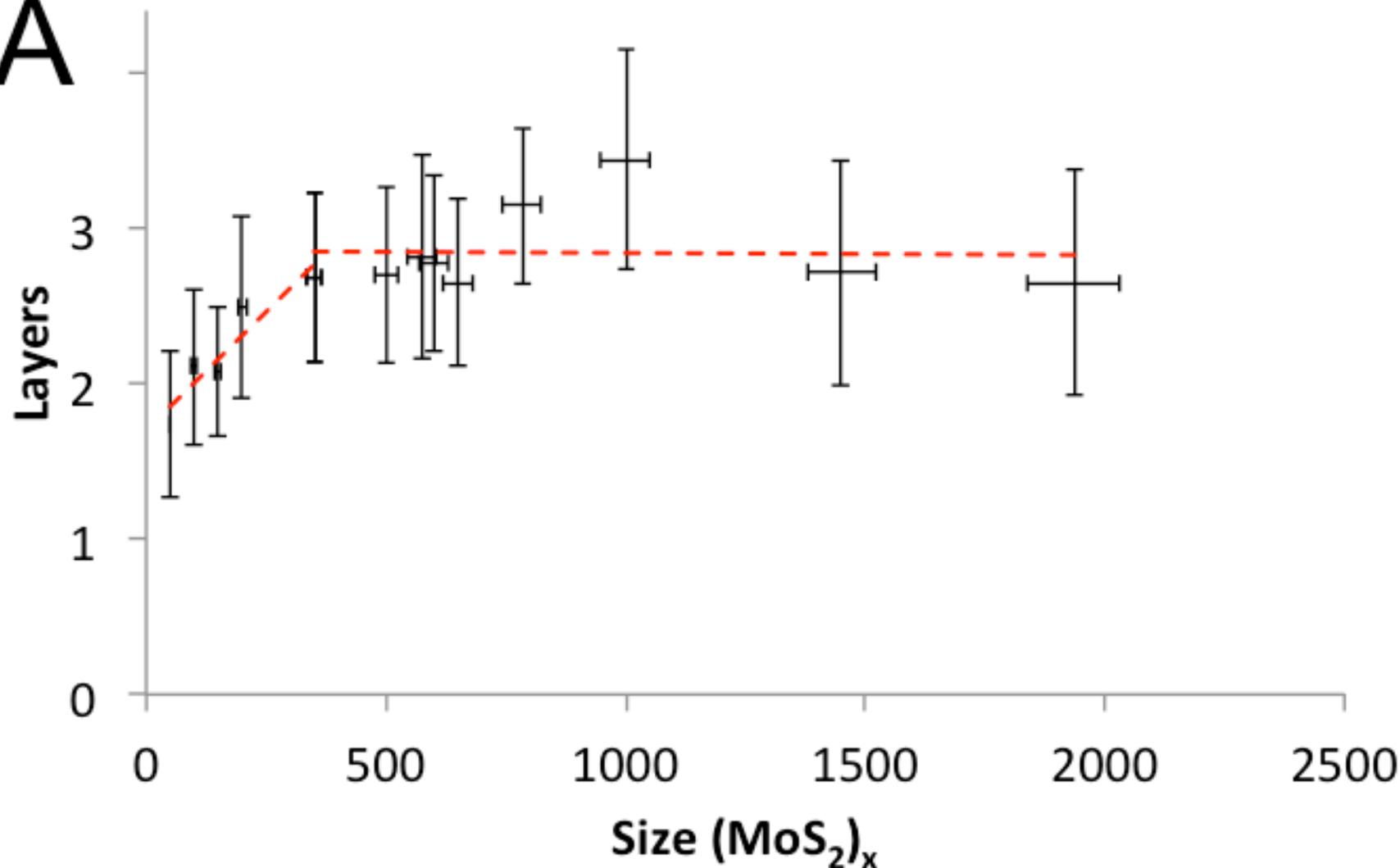
Layer height as a function of cluster size (derived from selected size + measured cluster footprint, both in MoS<sub>2</sub> units). The values derived are in agreement with observed line profiles from STEM micrographs.
