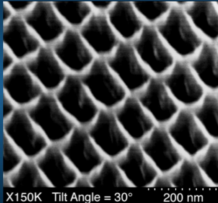
Grating in silicon; wall width is 20 nm and hole depth is 160 nm
