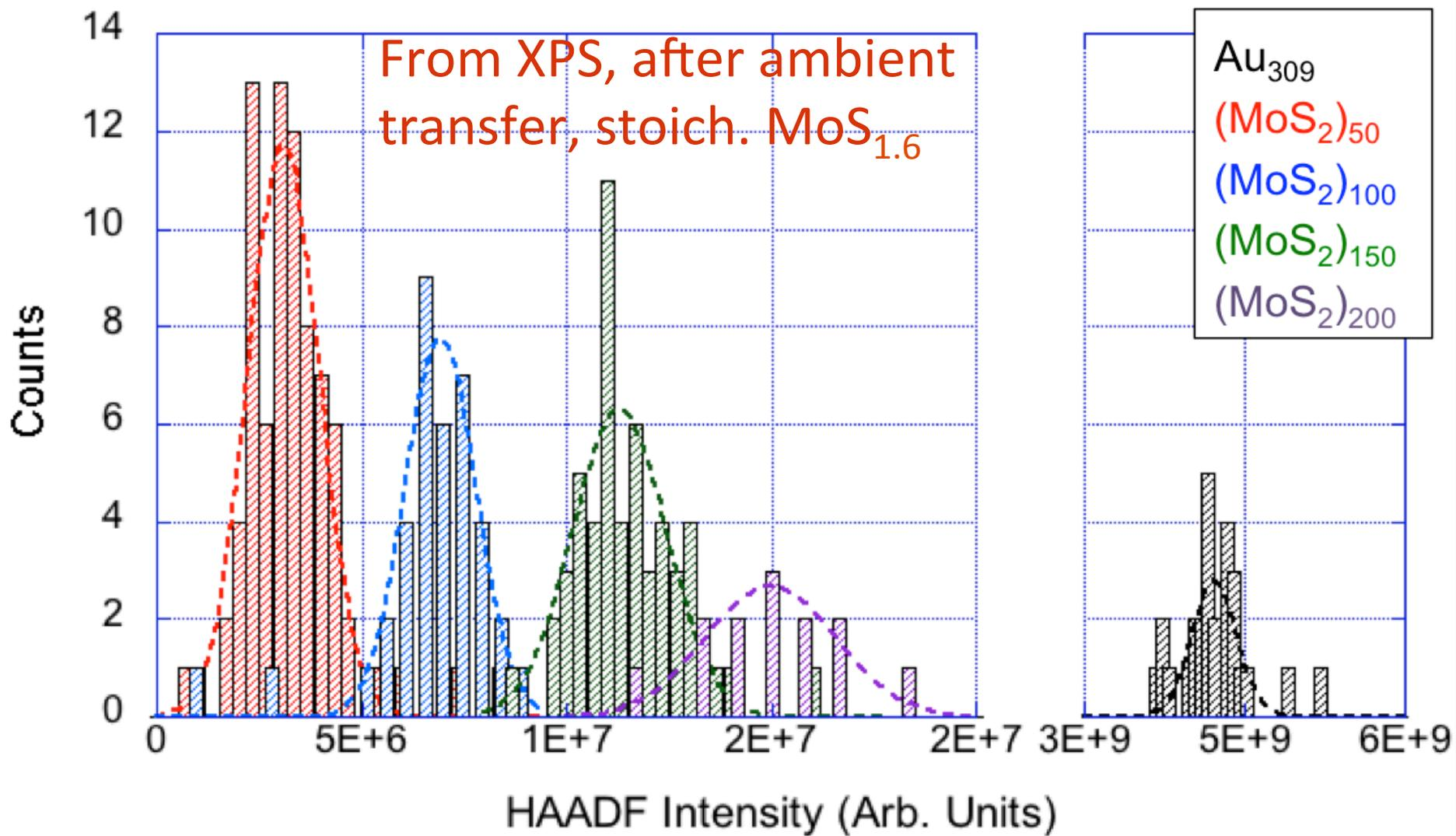
MoS<sub>2</sub> cluster and Au mass standard distributions, with Gaussian fits to negate the effect of outliers. FWHM of peaks,  $\delta m/m$ : Au<sub>309</sub>, 5.0%; (MoS<sub>2</sub>)<sub>50</sub>, 27.9%; (MoS<sub>2</sub>)<sub>100</sub>, 12.5%; (MoS<sub>2</sub>)<sub>150</sub>, 10.1%; (MoS<sub>2</sub>)<sub>200</sub>, 10.5%.
