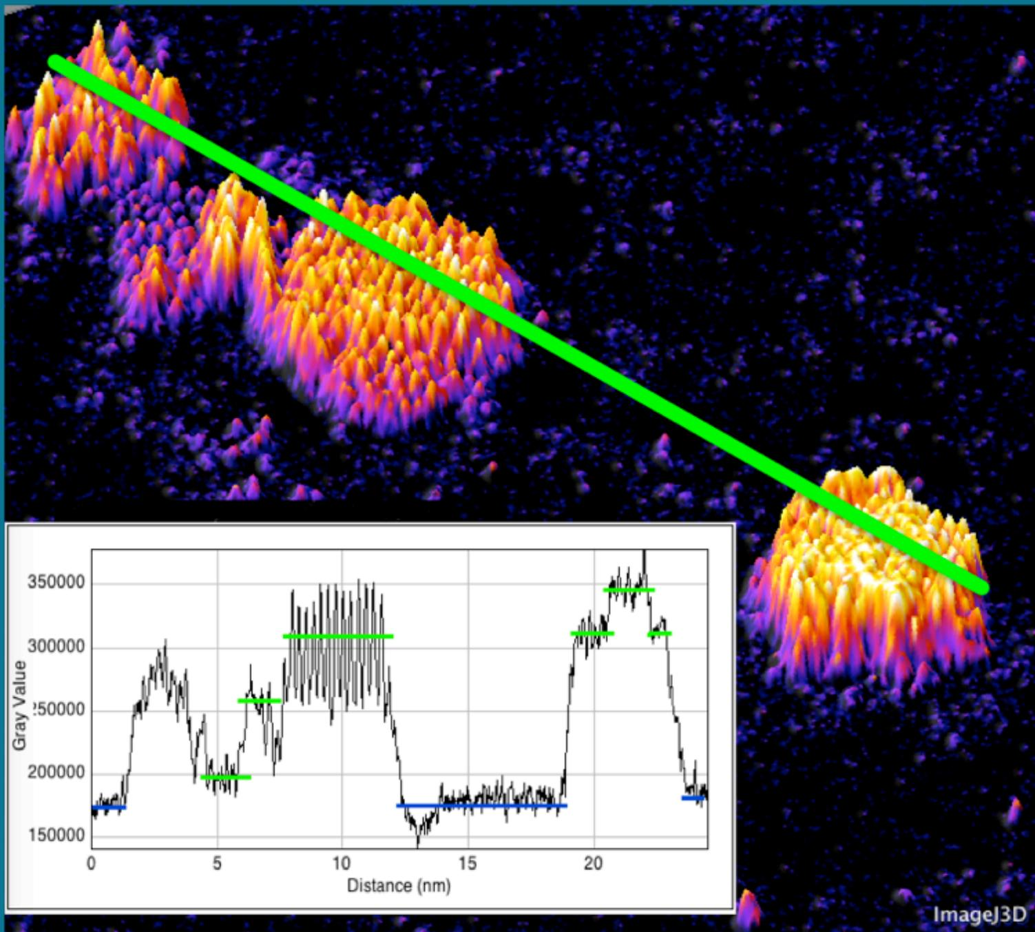
3D projection from a STEM micrograph of (MoS<sub>2</sub>)<sub>500</sub> clusters. (Inset) Line profile along the clusters showing layered structure (4 layers).
