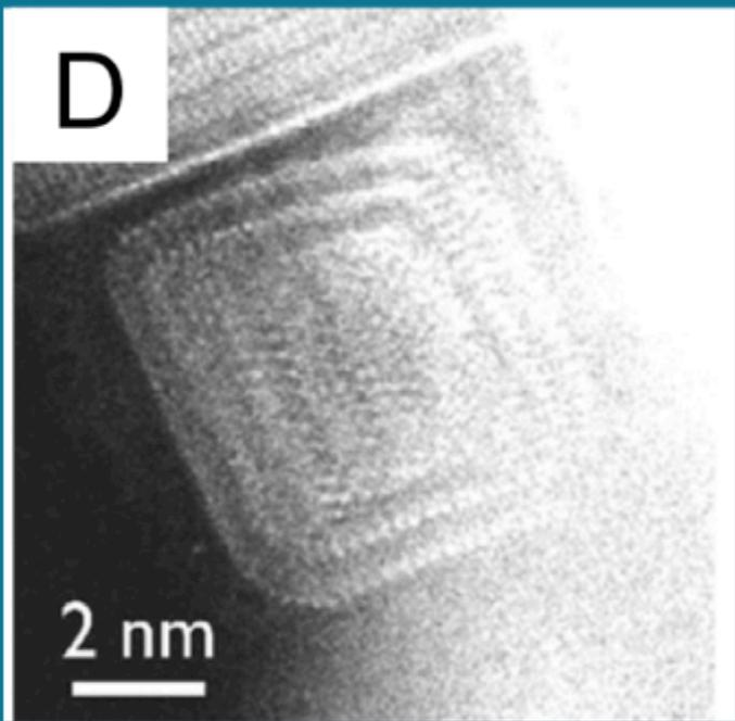
(A) STEM micrograph of seashell type ( $\text{MoS}_2$ ), compared with (B) a simulated seashell structure [1]. (C) STEM micrograph of ( $\text{MoS}_2$ )<sub>650</sub> fullerene candidate cluster and (D) other  $\text{MoS}_2$  fullerene clusters in literature [102].
