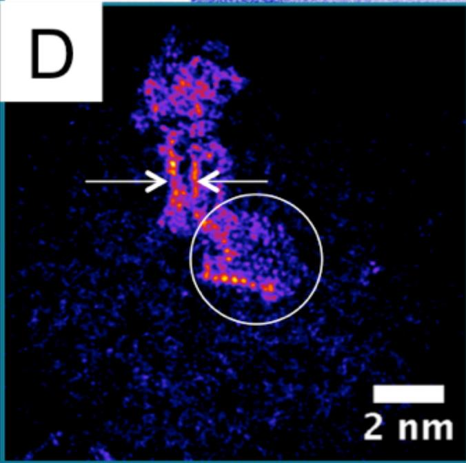
(A) (MoS<sub>2</sub>)500 trilayer and corresponding FFT (B) showing hexagonal crystal structure characteristic of bulk MoS<sub>2</sub> basal plane, with radial intensity profile highlighting the spots (B-Inset). (C) (MoS<sub>2</sub>)650 side-on showing basal plane edges (002) and (D) another (MoS<sub>2</sub>)650 with features from both (100) and (002) faces, probably assembled from smaller clusters in gas phase.
